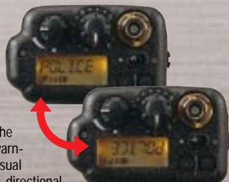
**PROGRAMMABLE TWO-COLOR LED** The two-color LED provides traditional transmit/ warning (red), receive (green), and alert (orange) visual indications. This LED is recessed to limit omni-directional visibility to everyone except the radio operator. If desired, the "green-busy" and "red-transmit" activities can be disabled independently for law enforcement or covert work.
